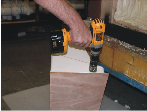
Figure 10. Drilling Hole for Cables
